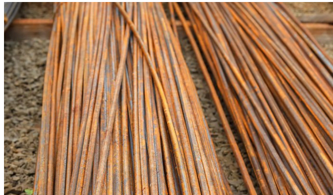
Fig 8. Corroded of reinforcing steels in open atmosphere before constructed (Web-8)
