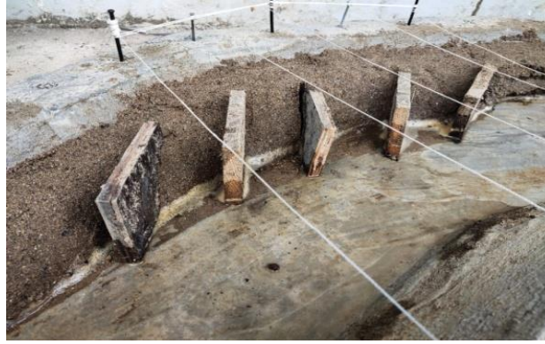
Figure 2: The Placement of the crib walls with slope angle of 60°
